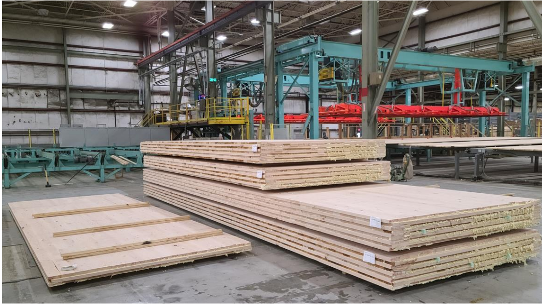
Eastern hemlock CLT panels manufactured at SmartLam, Dothan, Alabama – ready for cutting into testing smaller panels or “billets” to be shipped to the APA testing lab in Tacoma, Washington.
